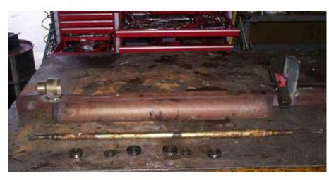
Note: before reassembly remove one of the seals from the bearing and repack with grease, This will extend the life of the bearing.
