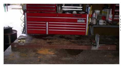
Toro 4500D roller bearing press. Roller can be disassembled in about 5 min. with a little heat. WITHOUT removing the end caps.
